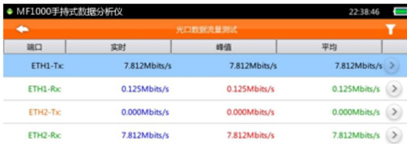
The screenshot shows the '光口数据流量测试' (Optical Port Data Traffic Test) interface on an MF1000 handheld data analyzer. The interface displays a table with four columns: '端口' (Port), '实时' (Real-time), '峰值' (Peak), and '平均' (Average). The data is as follows:
